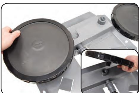
3. Screw diffuser(s) onto 3/4" FPT on top of unit. Snug fitting by hand. **Do not over tighten.**
