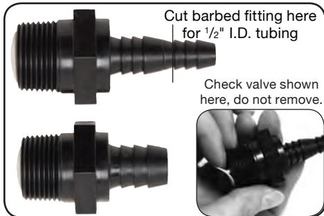
1. 3/4" MPT barbed check valve is designed to be used with 1/2" or 5/8" I.D. tubing. Use larger barbed fitting for 5/8" ID tubing
