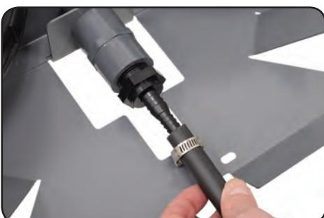
4. Use supplied hose clamp, slip loosely over end of tubing and push tubing tightly onto the fitting.
